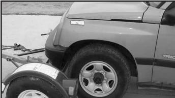
**Step 5.** With someone safely guiding you, slowly drive vehicle onto platform **FRONT FORWARD.** (Any vehicle mounted on tow dolly must be mounted with front of the vehicle facing forward.) Drive the car forward until the tires touch the ramps. Make sure the tire is aligned to ascend onto the ramps.
